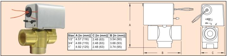
**3ZV1 Series Zone Valves are ideal for flow control** in hot and cold water HVAC systems. The 3ZV1 is electrically driven to open and spring to close. Units are available in 1/2", 3/4", and 1" sizes with 24 or 120 VAC power supply. Easy to install these units are direct replacements for competitor units. Manual override lever is easily accessible externally. Consult factory for 220 VAC power supply, optional auxiliary switches, and BSP or sweat connections.
