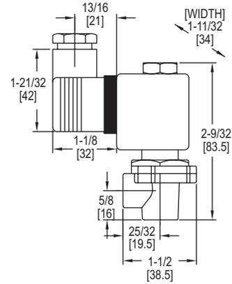
The **Series RSV Pilot Solenoid Valve** is used to operate the Series RDCV remote type diaphragm valve to air pulse clean filters in dust collectors. Consult factory for mounting of RSV valves with our DCT timer boards together in one enclosure all pre-wired.
