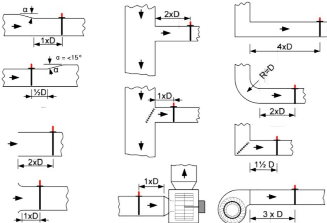
D = duct diameter or equal diameter
